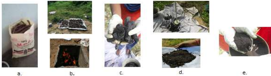
Fig 01. a. koonka (palm flowers), b. koonka being sundried and 3/4 th burning of the sundried koonka, c. charcoal burning of koonka, d. grinding of charcoal and powdered charcoal (before sieving) and e. charcoal powder after sieving
